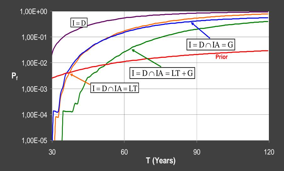
I: Inspection, D=Detection IA: Invasive Action, LT=Load Truncation, G=Weld Toe Grinding
